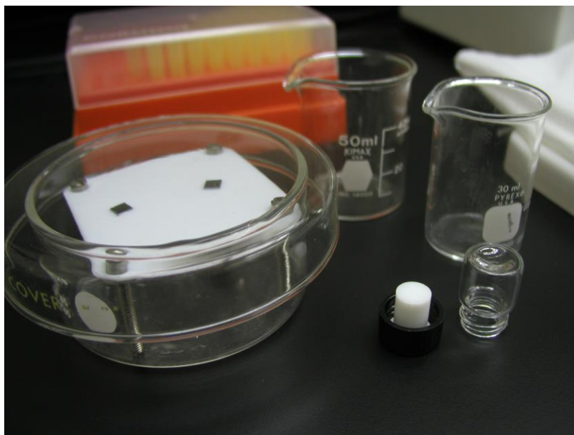
Figure 1. Apparatus used to functionalize and capture nanoparticles on TEM grids. Shown are the small glass vial with Teflon pedestal in the inverted cap, Teflon block with two test chips under cover, beakers used for dip rinsing, and a box of pipette tips.
